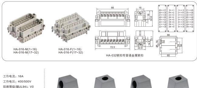
阻燃等级(据UL94): V0 防护等级:IP65 接线形式:螺钉压接 弹片压接 电缆入口可选螺纹: PG21, PG29 Rated current: 16A Rated voltage: 400/500V Flammability acc. to UL94: V0 Degree of protection acc. to DIN40 050: IP65 Terminal: Screw terminal Spring terminal Thread: PG21, PG29
